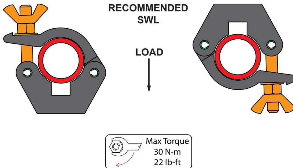
THE FOLLOWING APPLICATIONS WILL RESULT IN THE RECOMMENDED SWL BEING REDUCED DEPENDANT ON THE TUBE SURFACE FINISH & TORQUE SETTINGS APPLIED. PROOF LOADING ON INSTALLATIONS IS RECOMMENDED.
