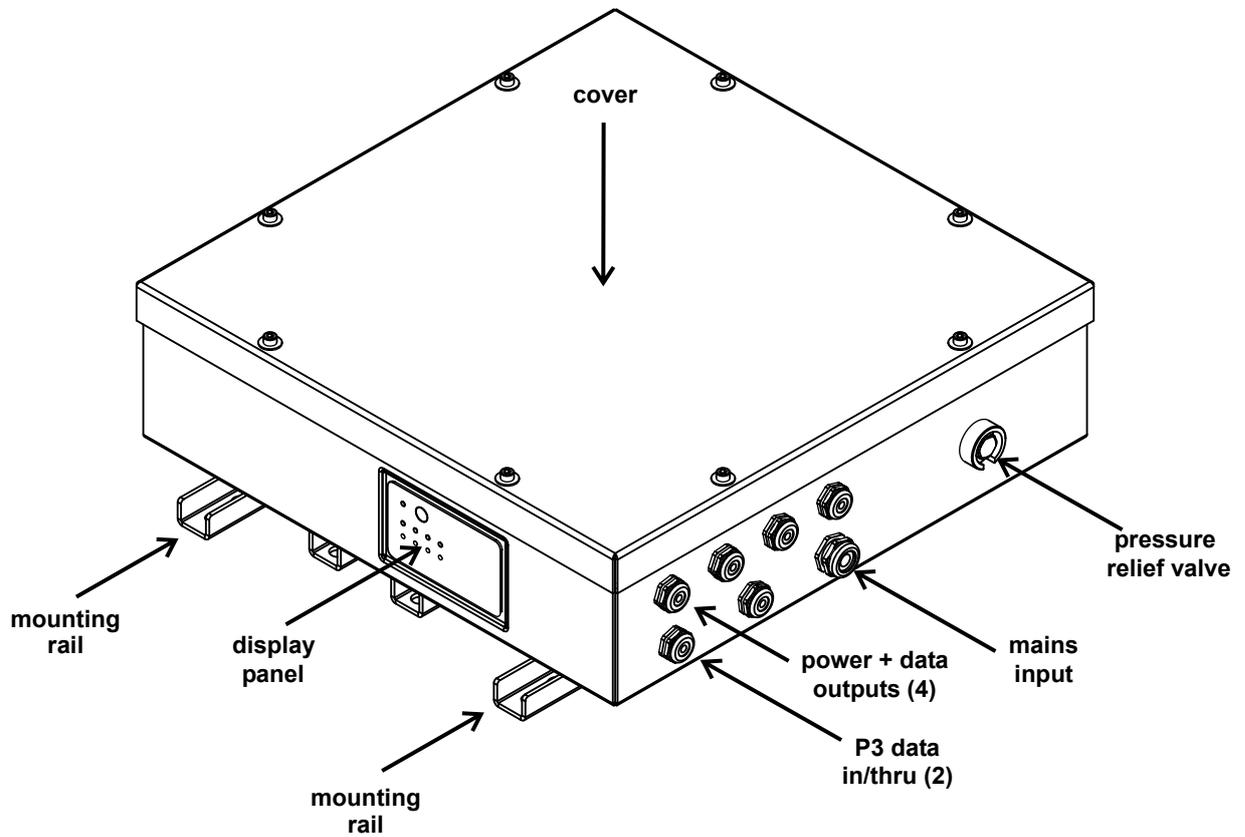
Figure 1: Parts identification
