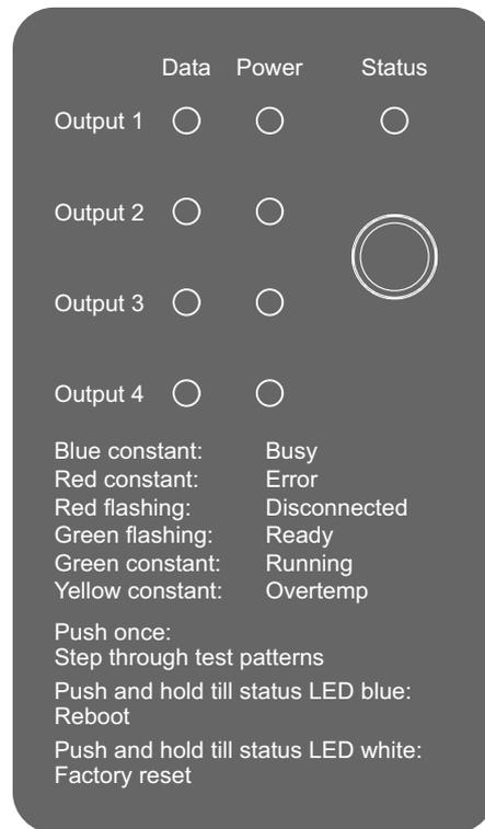
**Figure 7: Status LEDs and control button**
