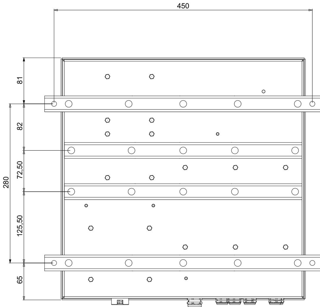
**Figure 4: Mounting hole spacing (in mm)**
