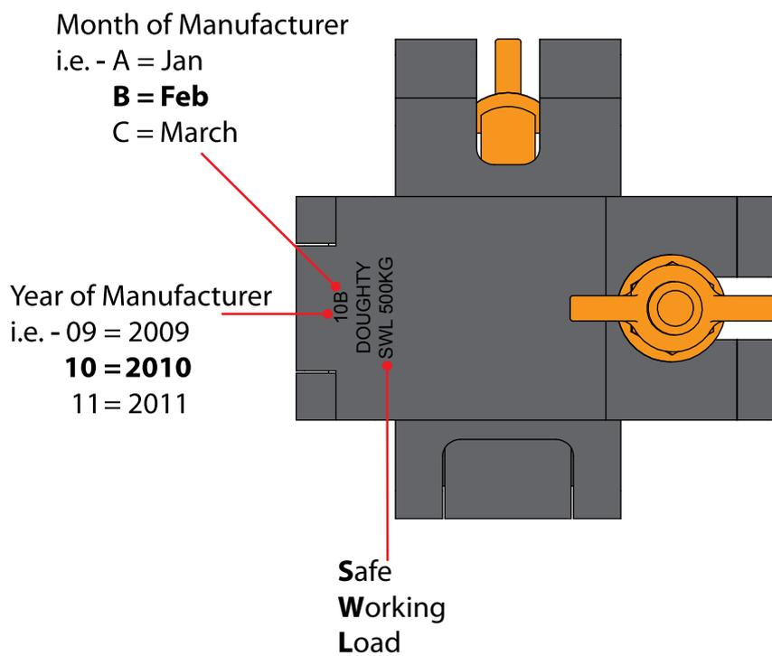
1. Never exceed the Safe Working Load (SWL) shown on the clamp.
