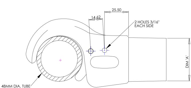
NOTE; 3/16" HOLE POSITIONS IN THIS VIEW ARE APPLICABLE TO DIA. 48 BARREL ONLY
