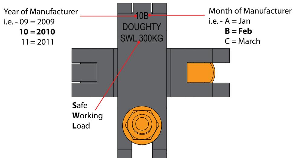
1. Never exceed the Safe Working Load (SWL) shown on the clamp.
